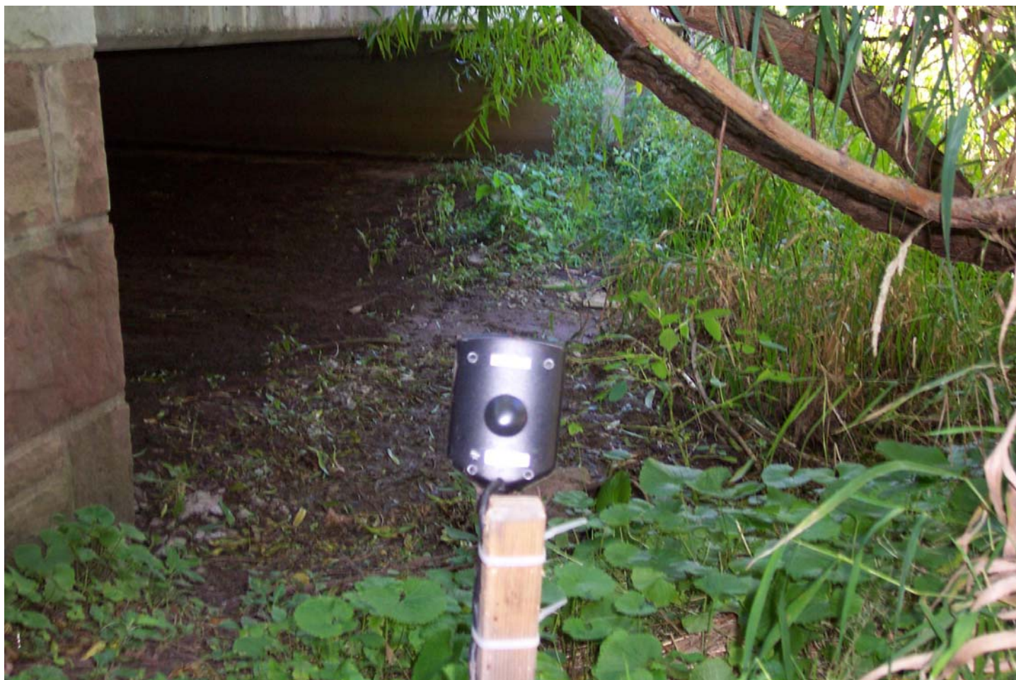
Figure A-1c. Back view of a MustelaVision camera head mounted on stake at the Round Pond Creek site in the BBWMA.
