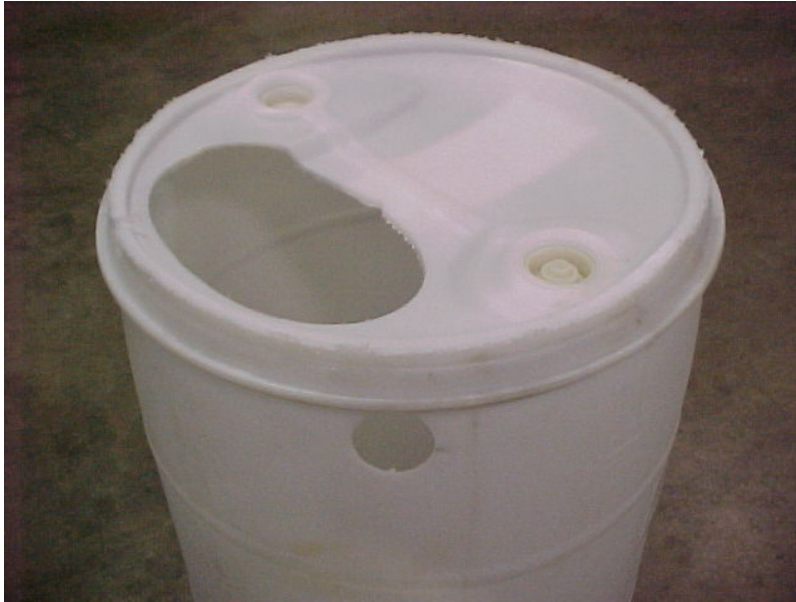
Inverted cover with inflow and drainage hole, and overflow hole on side.
